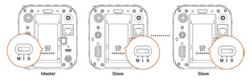
2. Plug the LEMO end of the Sync Cable into the I/O port on the rear of the camera. Use a cat 6 Ethernet cable to connect the Output end of the Master camera Sync Cable to the Input end of 1<sup>st</sup> Slave camera Sync Cable. Then connect the Output end of 1<sup>st</sup> Slave camera Sync Cable to the next Slave camera Sync Cable Input end. So on and so forth, for the rest of the slave cameras.
